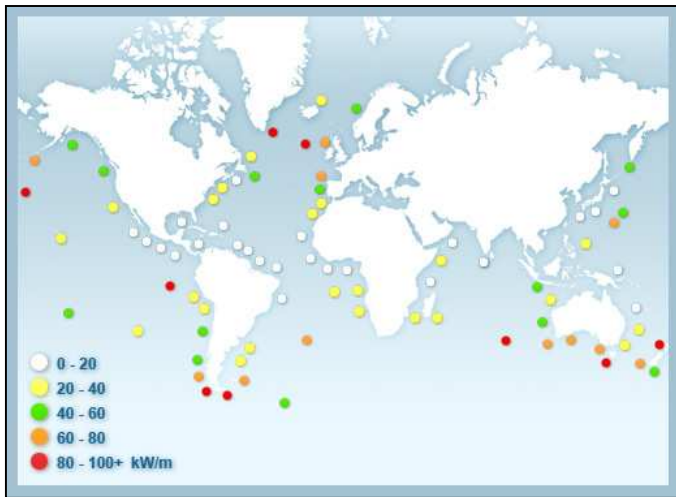
Figure 1: Density of wave power (source: www.aw-energy.com)
